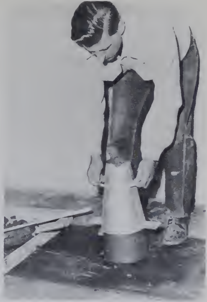
Slow, steady, vertical removal of the mold
